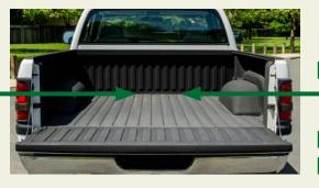
Full-Size Pickup: 5ft X 7ft Bed Filled to top of bed = 1.33 cubic yards Filled to top of cab = 3.89 cubic yards
